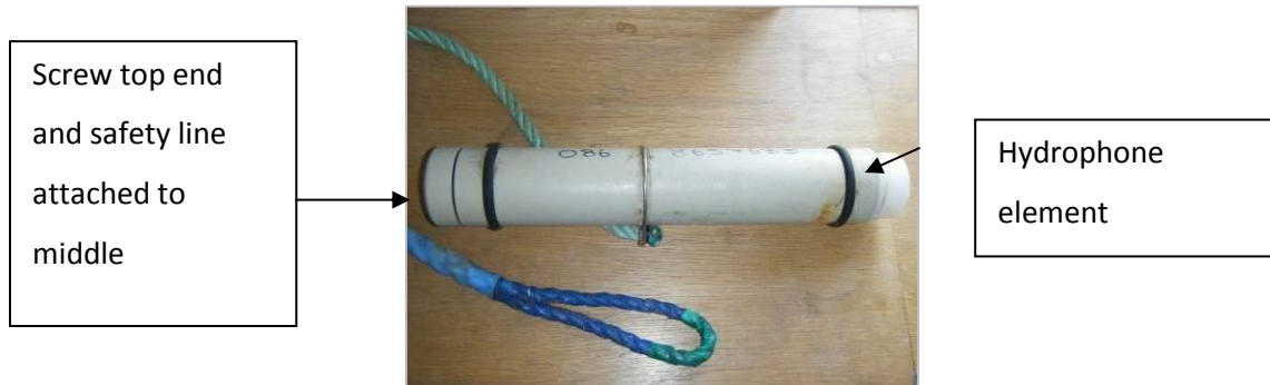
Figure 5. C-POD unit by Chelonia Ltd
